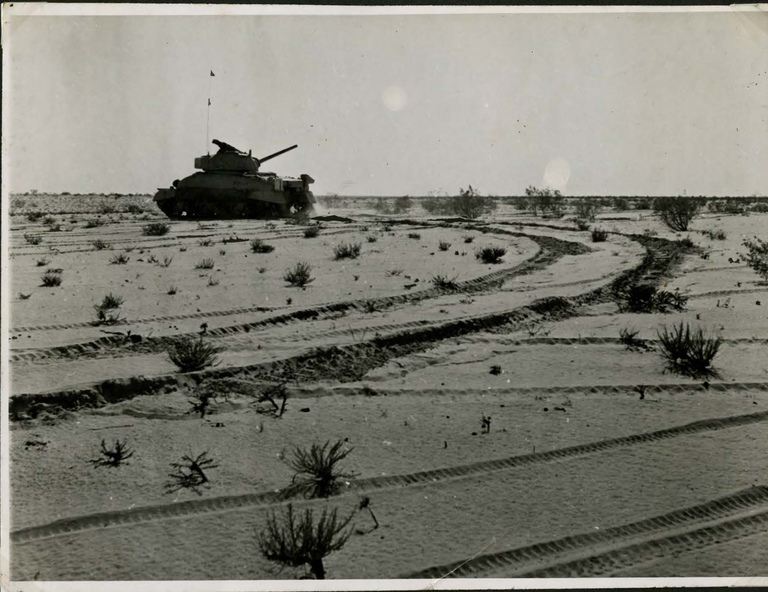
A Sherman tank. The turret had a 360° traverse. A 75m.m. gun. Weight - 30 tons. Price: -£30,000.
