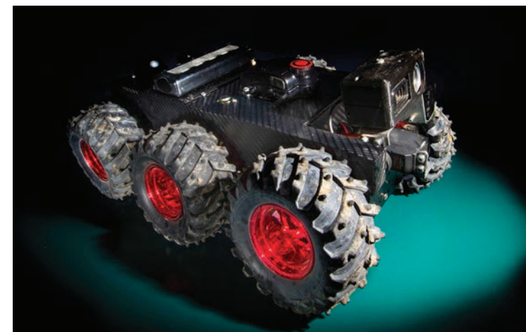
The Techmatics robot which can remotely inspect the foundations of houses.
